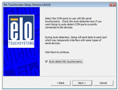
The following window appears. The touch panel connected to the ST-A20 and the TFTST-A20 are detected, and "COM6" and "COM1 or 2" are chosen. If "COM6" and "COM1 or 2" is not chosen, there may be a problem. Click on the "Next" button.
