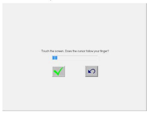
The following calibration screen appears on TFTST-A20 screen. Perform a calibration by touching the mark whenever it appears. (The mark appears three times.)
