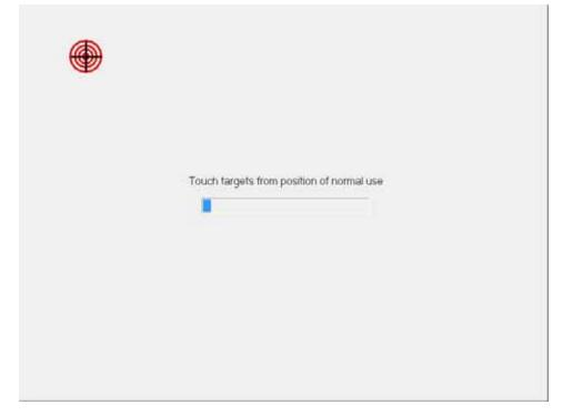
After the mark was touched three times, two buttons appear at the center of the screen. Click on the check mark button to complete the calibration
